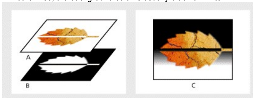
A. RGB image as it appears in original application B. Alpha channel in original application C. Image correctly displayed as premultiplied with white in After Effects
