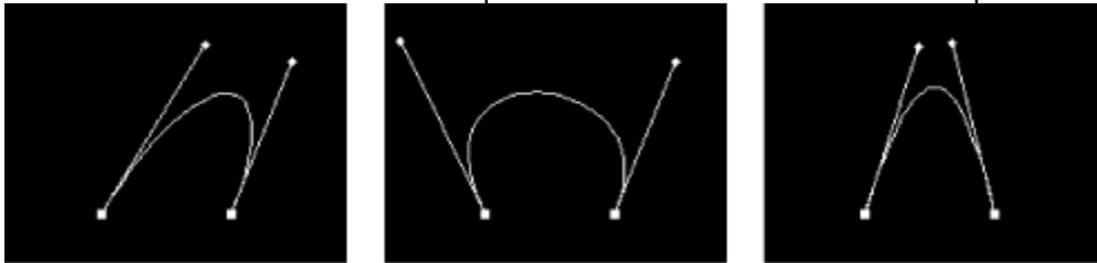
Moving a direction line changes the slope of the curve
